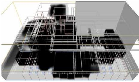
Fig. 14. Smoke movement at 40s.
