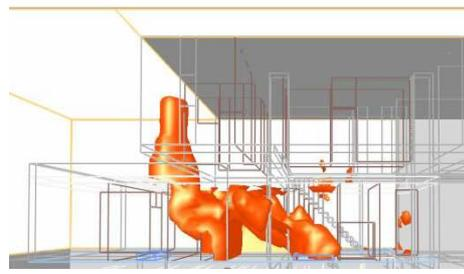
Fig. 15. Fire spread at 300s.
