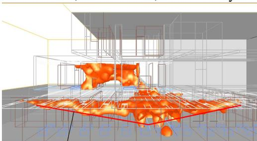
Fig. 12. Fire spread at 40s.
