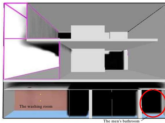
Fig.18. Inability of smoke spreading into the men's bathroom where 1 man survived.
